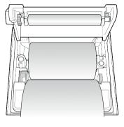
6.5 Close the lid and make sure that the paper is positioned between the lid and the front of the printer
