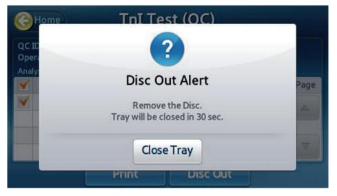
Press the Home button or the Disc Out button to open the tray. Remove the disc and discard appropriately.
