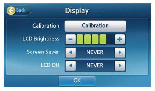
A screen saver turns on to protect the display when the screen has not changed after a specified length of time.
