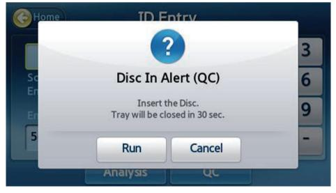
When the tray opens, insert the control disc or EQC disc into the tray and press Run.
