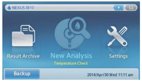
**T**est is limited if the analyzer is out of operational temperature range.
