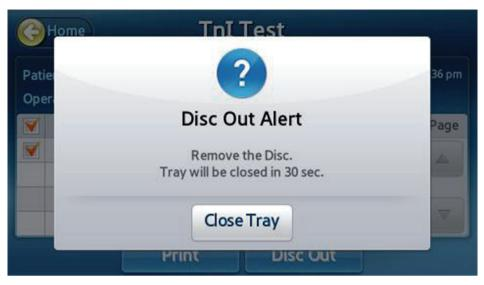
After the test is complete the tray will open. Remove the disc and discard appropriately.
