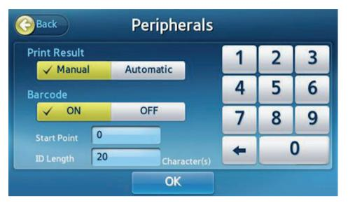
The analyzer can be set to automatically or manually print test results.
