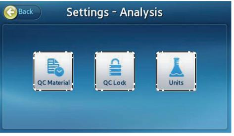
Press Analyze on the Settings screen to change QC Material, QC Lock, and the Units settings.
