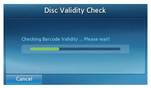
When the tray closes, the analyzer performs a disc validation, and will display the name of specific disc being tested.
