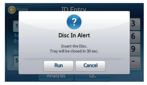
When the tray opens, insert a disc loaded with a sample into the tray and press Run. Disc Validation and Starting Test
